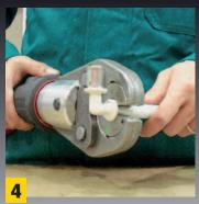
Open the jaw and introduce the fitting into them. Perform the pressing operation and pay attention that the bushing is centred.
