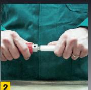
After calibration, a 1mm-deep ream around the pipe must be visible. It is recommended to perform this operation ONLY with original aquatechnik tools.
