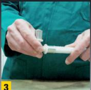
Introduce the pipe into the fitting up to the end point. It is visible through the specific control holes that are to be found in the steel bushing. Only a well-done assembly assures the perfect sealing of the connections.
